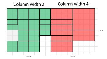
Fig. 7. The atlas is divided into square superblocks (8x8 in the figure). The green superblock is subdivided into columns of width 2, and the red superblock is subdivided into columns of width 4. Columns are packed with blocks of variable height.
