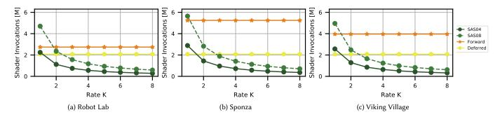
Fig. 12. Comparison of fragment shader invocations (in millions) for forward rendering, deferred rendering and standalone object-space shading with our Shading Atlas. The x-axis displays the upsampling factor K, describing how many frames are generated from a single shading atlas.
