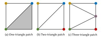
Fig. 4. Our system supports three different patch types with one, two or three triangles. The preferred patch type is the two-triangle patch.
