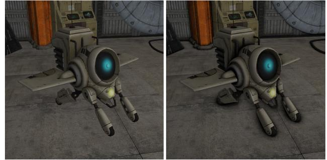
Fig. 17. To demonstrate how postprocessing effects can be integrated into SAS, we added screen-space ambient occlusion to the shading stage. The screenshots show Phong shaded images without (left) and with (right) SSAO.
