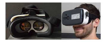
Fig. 9. Untethered smartphone-based headset prototype based on the Qualcomm Snapdragon  $^{TM}$  835 Mobile Platform, with a resolution of  $2560 \times 1440$ , displaying a stereo view of the Robot Lab scene.
