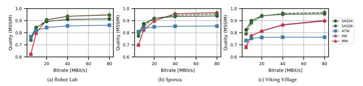
Fig. 15. Rate distortion curves after MPEG compression. We report image quality (MSSIM) as a function of network bitrate for SAS (using multiple atlas sizes), asynchronous time warping (ATW), mesh warping (MW) and iterative image warping (IIW).
