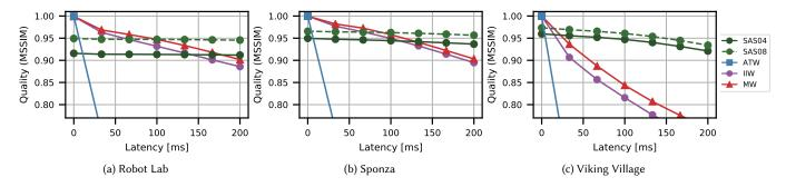
Fig. 13. Image quality (reported as MSSIM) for varying network latency, compared for SAS (using multiple atlas sizes). As latency increases, SAS maintains image quality better than asynchronous time warping (ATW), mesh warping (MW) and iterative image warping (IIW).
