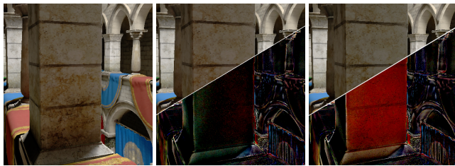
Figure 4: Comparing the accuracy of color bleeding in the final image. While SST (b) faithfully captures the soft reflection of the red fabric on the pillar as it is seen in the ground truth (a), it is almost entirely missing with SLC (c). The bottom right half of (b,c) shows the pixel difference \times 10 .
