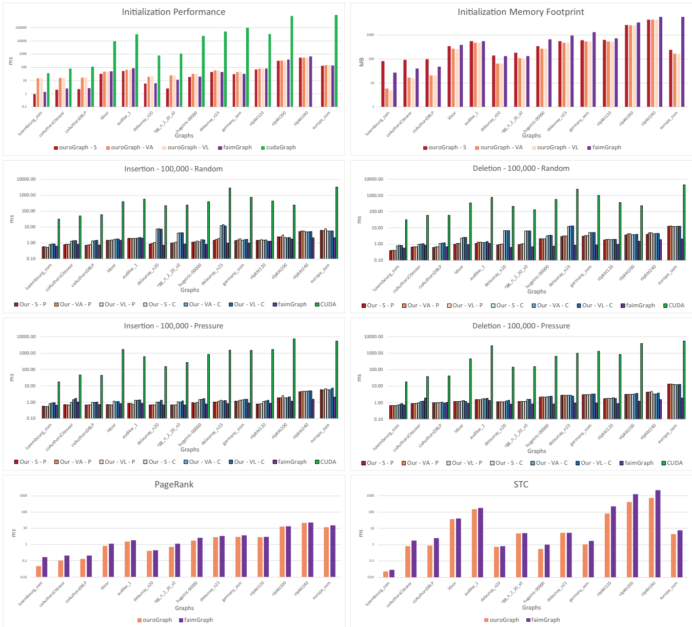
Figure 4: Dynamic graph performance for OuroGraph variants ( S | VA | VL denote standard, virtualized array-based and virtualized linked-list based methods, P | C define if page or chunk indices were stored), faimGraph and CudaAllocGraph . Top Left: Initialization performance for given graphs in ms, Top Right: Memory footprint after initialization in MB, Middle: Two test-cases, updating 100 000 edges with randomized source (second from the top) and 100 000 edges with source focused on a range of 1000 (third from the top), insertion performance on the right and deletion performance on the left. Bottom Left: Algorithm performance for PageRank and Bottom Right: Algorithm performance for STC.
