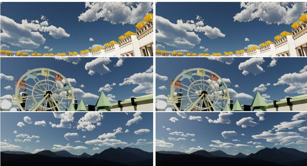
**Figure 7:** Visual comparison between screen space (left) and our view cell-based caches (right) at various offsets (from top to bottom 6m, 300m, 2000m) to the view cell's location. The first two image pairs only show a small positional error of the clouds which is not noticeable. Whereas in the third row, the clouds are visually distorted towards the view cell center and start to look flat.
