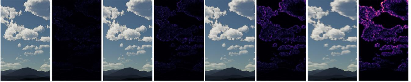
**Figure 8:** Quality comparison between different mip bias settings showing pairs of the final image and the calculated FLIP error compared to the screen space implementation. The pairs from left to right correspond to the following mip biases [0, 1, 2, 3]. With a mip bias less or equal to 1, barely any difference is noticeable. With a mip bias of 2, the FLIP error starts to show more noticeable differences, which were not detected by our user study participants (Q1).
