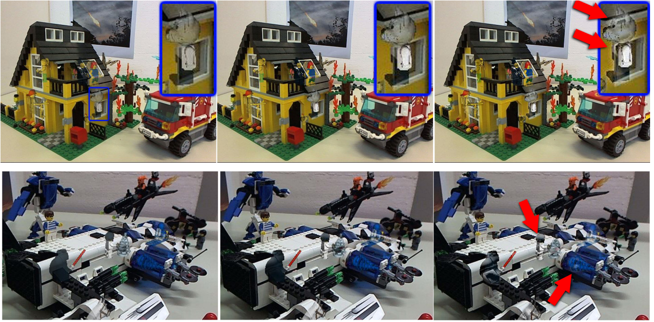
Figure 6: Experimental scenes from the first study. We compare alpha blending (left) and common ghosted views (middle) with emphasized ghosted views (right) in scenes with conflicting visual characteristics. Notice the emphasized structure covering the virtual objects marked with red arrows in the lower row and the emphasized structure within the enlarged inset in the upper row.
